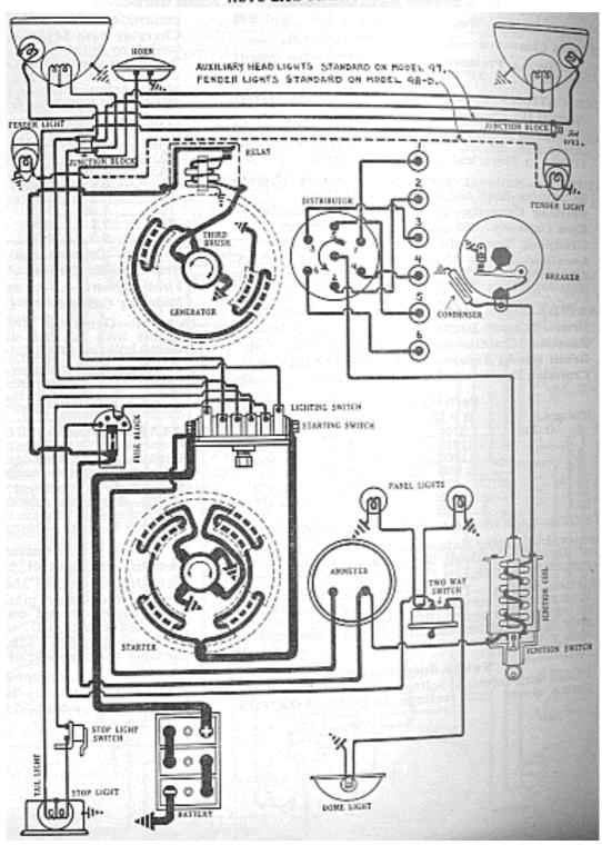
BATTERY:-U.S.L., Type XY-13X-7A, 6 volt. The negative (-) terminal is grounded. Starting capacity (20 minute rate) is 102 amperes for 20 minutes. Lighting capacity (5 ampere rate) is 5 amperes for 17.6 hours. Battery is mounted under the front compartment floor boards on the left side.
