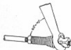
Fig. N19. Correct angle of Bendix levers with brakes released
