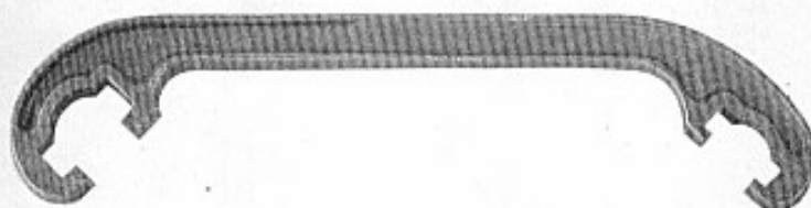
Fig. N24—16-in. double-end box wrench for Bendix anchor nut. Proper tightening of anchors requires 16-in. leverage
