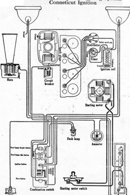
Battery.—Battery is 6 volt, 80 ampere-hour. The negative (—) terminal is grounded at the starting motor.
