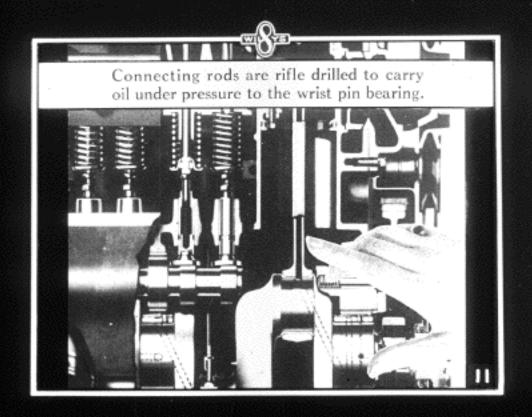
Thoroughness of Lubrica tion is typical of Willys -Overland's thoroughness of design-even the timing chain is lubricated under pressure.
