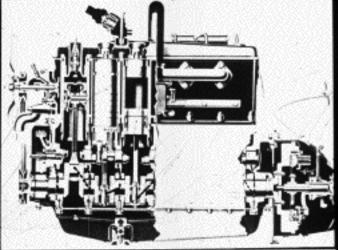
Pressure lubrication to all crankshaft, connecting rod and eccentric shaft bearings also maintains quietness and long life over the years.
