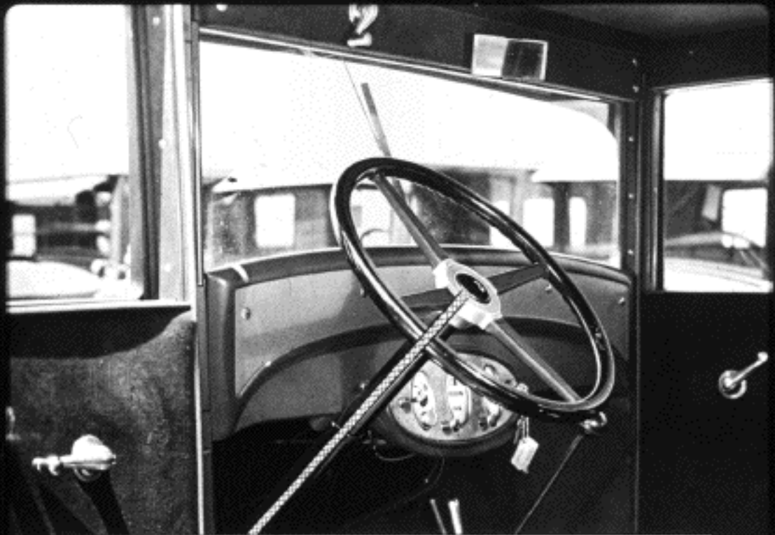
The Superior Whippet's Finger Tip Control has likewise done away with horn or light wires in the steering post.
