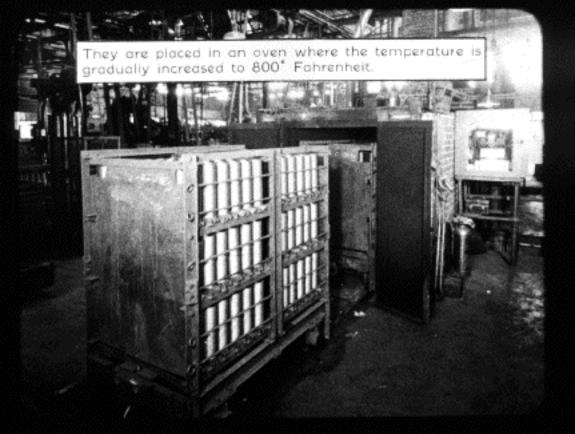
This intense heat is maintained for a period of time after which the sleeves are gradually cooled before they are removed from the furnace. Following the annealing process the sleeve goes through a semi-finish reaming operation which straightens up the inside bore.
