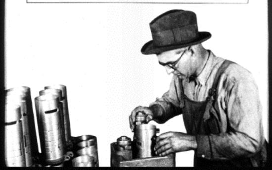
proper dimensions and alignment of sleeve rod lug and alignment of the bore. The inside diameter of the sleeve must not vary 5/10,000 of an inch or 1/4 the thickness of the average human hair if it is to pass the inspection.
