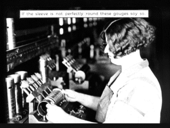
After checking four or five sleeves the inspector checks his gauges with a standard true cylinder.
